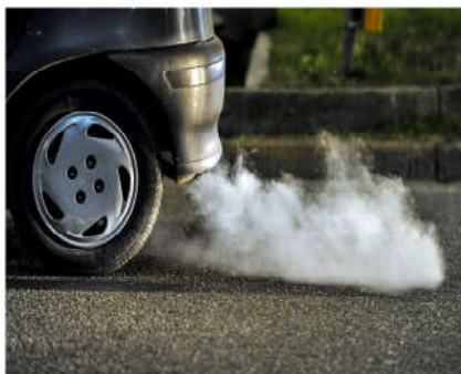
WRONG FUNCTION-turbocharger connect to diesel particulate filter
